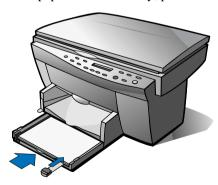
3 Slide the paper width and length adjusters in until they stop at the edges of the paper.
